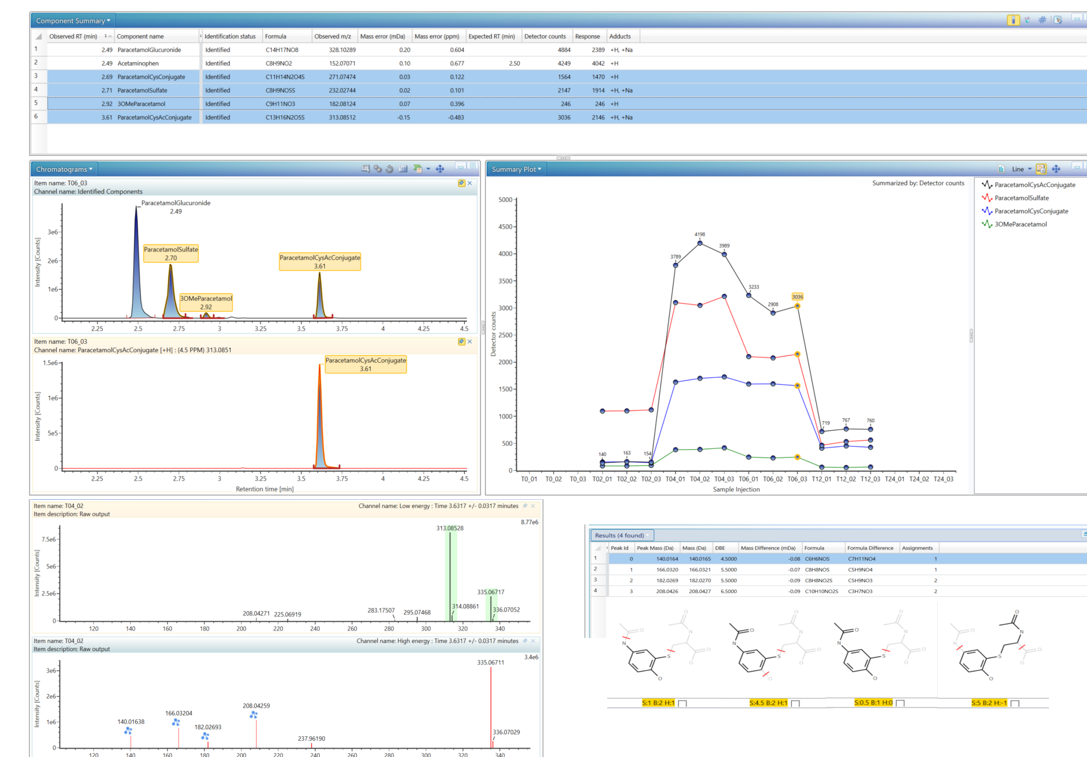
Figure 9. Study of in vivo metabolites of Paracetamol. Metabolites present at 4 hours were identified using accurate mass measurement and fragmentation patterns. The average mass error for the identified metabolites was 0.236 ppm with an RMS error of 0.454 ppm. Timecourses for metabolites are shown, matching established pharmacokinetics for Paracetamol excretion. MS E Low and High energy spectra for the Acetylcysteine conjugate of paracetamol along with MassFragment report of assigned fragment ions and mass errors.
