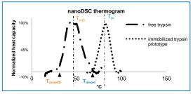
Figure 1. NanoDSC thermograms of free trypsin and one optimal immobilized enzyme prototype.
