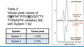
Figure 2. %base peak value is one of the criteria (thresholds) used in new peak detection. It is calculated relative to the intensity of the most abundant peptide of the chromatogram. The System 2 shows high %base peak values due to improved recovery of peptides. An example peak eluting at 62.89 min (D<u>MIFNFYFDV<u>W</u>GQGTTVTVSSAS TK) in stressed sample of NISTmab is shown here</u>
