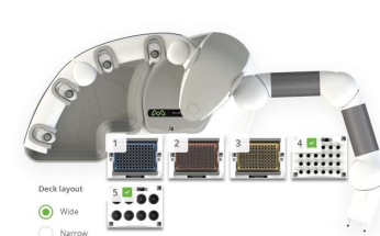
Figure 2 Andrew+ deck configuration for the triptorelin working solutions preparation protocol.
