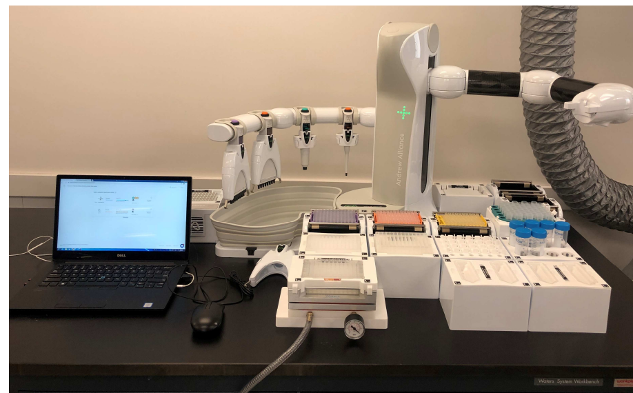
Figure 2. Andrew+ Automation Workflow Setup for Oasis 2x4 Method Development
