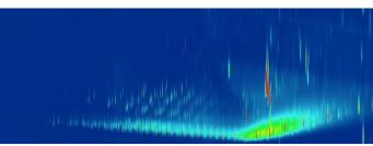
The limitations of 1D GC (above, left; 1D projection of biodiesel) are made clear and are demonstrated through unresolved peaks and coelution. However, the 2D heatmap projection (above, right) shows all of the peaks that have been resolved in the second dimension. This capability can be extremely powerful for complex matrices.
