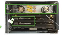
Two pumps Two identical flow paths Two identical columns
