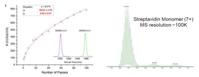
Ion Mobility resolution is scalable by selecting the number of cycles of IMS separation, with IMS resolution  $(\Omega/\Delta\Omega)$  increasing as the square root of the number of cycles . 100 IMS cycles generates ~800 IMS resolution, with an ion signal loss of only ~1% per cycle. TOF Detection can be acquired with selectable MS resolution of 60,000 (V-Optics) to 100,000 (W-Optics).
