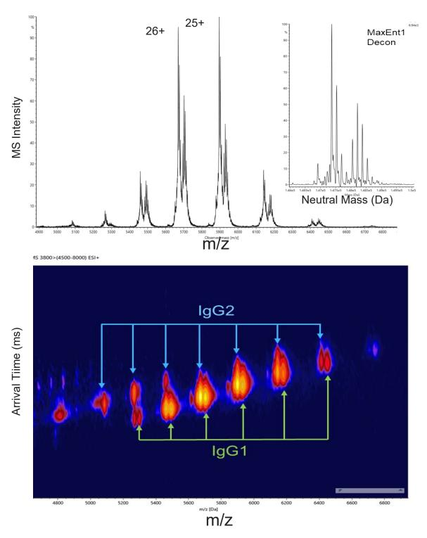
Co-infusion of an IgG1 and IgG2 molecule generates a mass spectrum and deconvoluted mass spectrum (TOP Panel) with largely resolved component signals. One IMS Cycle revealed (BOTTOM Panel) a single structural form for the  $IgG_1$  and two major structural forms for the  $IgG_2$  molecules.
