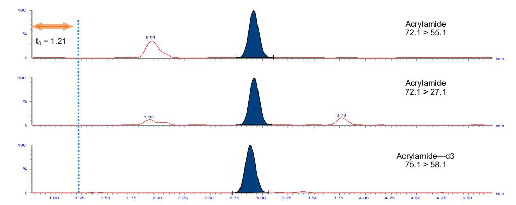
**Figure 4.** Chromatogram of an extracted, FAPAS coffee reference sample, measured at 244 μg/kg. The t<sub>0</sub> of the column ran at the 0.2 mL/min flow rate is indicated on the chromatogram, highlighting the **excellent retention** achieved with a simple LC gradient.
