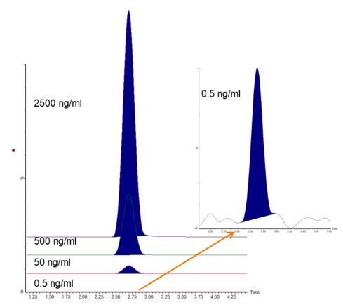
**Figure 3.** Example of quantifier ions achieved for the calibration range in Figure 2, thus showing excellent sensitivity and linearity (without saturation) over an extended **concentration range**.
