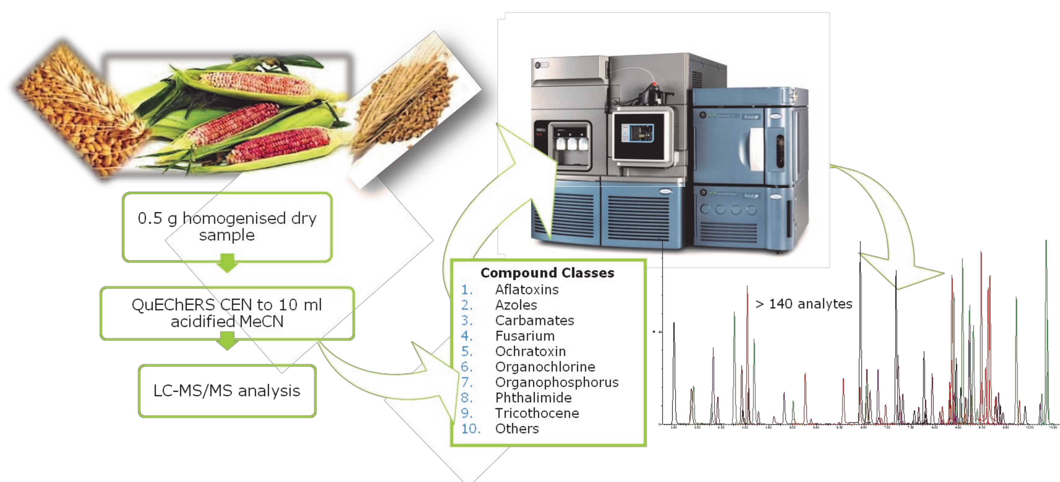
Figure 2. Generic, single step QuEChERS clean up was applied to samples of barley, red corn and wheat, spiked with over 140 analytes (including mycotoxins and pesticides) and presented for LC-US-MS/MS analysis.
