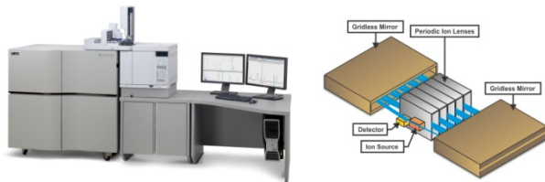
Figure 2. LECO Pegasus GC-HRT with Folded Flight Path (FFP) Technology.
