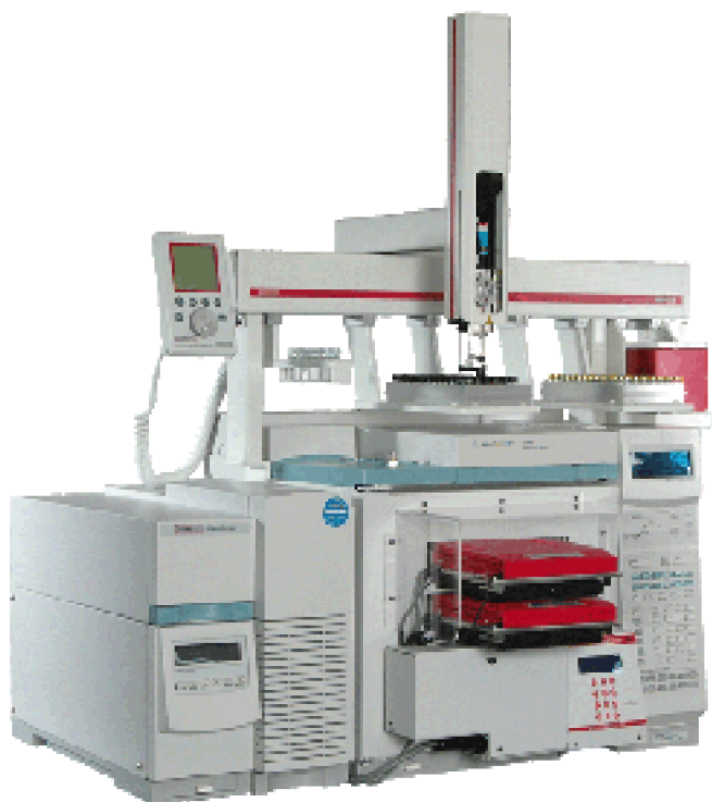
Figure 1. Dual Column MACH Connected to 6890 GC System.
