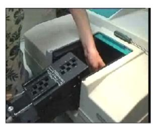
**Figure 2.** Resting the Multicell Holder accessory on the edge of the instrument. Note that the  $6 \times 6$  Multicell Holder is pictured, however the installation procedure is the same for the  $8 \times 6$  Multicell Holder.
