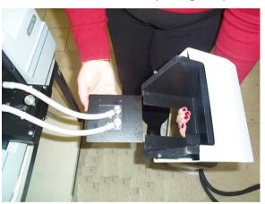
Figure 6. Slotting the accessory baseplate into the Extended Sample Compartment
