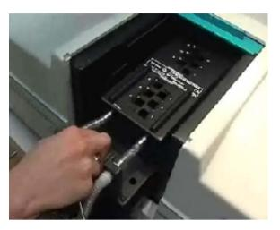
**Figure 5.** Sliding the top half of the accessory forward. Note that the  $6 \times 6$  Multicell Holder is pictured, however the installation procedure is the same for the  $8 \times 6$  Multicell Holder.
