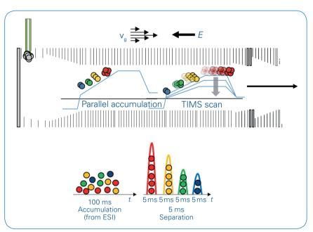
Figure 2: Confinement and release of the ions within the tims cell. All ions accumulated for 100 ms are concentrated in 5 ms width Ion Mobility Separated peaks, ensuring a dramatic increase in both acquisition speed and sensitivity. The dual tims cell architecture allows for parallel accumulation with close to 100% duty cycle: ions are still accumulated in the first cell as they are released from the second cell.
