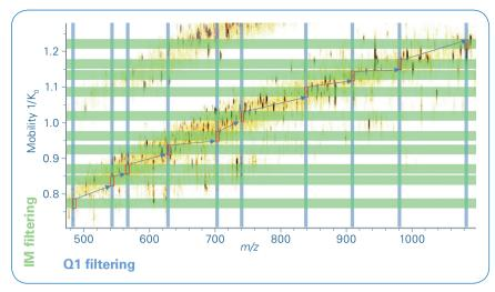
Figure 3: Selection of the targeted peptide precursor ions during a single prm-PASEF event. Several precursors can be selected within a 100 ms IMS scan and consecutively fragmented in the collision cell. High selectivity in the precursor's selection is obtained by combining the ion mobility (green bars) with the quadrupole isolation windows (blue bars)
