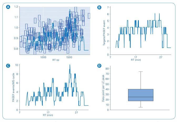
Figure 5: Illustration of multiplexing capacities. (A) Distribution of the 216 target windows in the retention time and ion mobility dimensions. (B) Number of distinct targets measured in parallel in each prm-PASEF frame. (C) Number of prm-PASEF frames required to cover all co-eluted compounds. (D) Number of data point / LC peak, for all targeted compounds.
