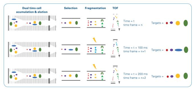
Figure 4: Distribution of compounds co eluted both in the retention time and ion mobility dimensions in two distinct prm-PASEF frames
