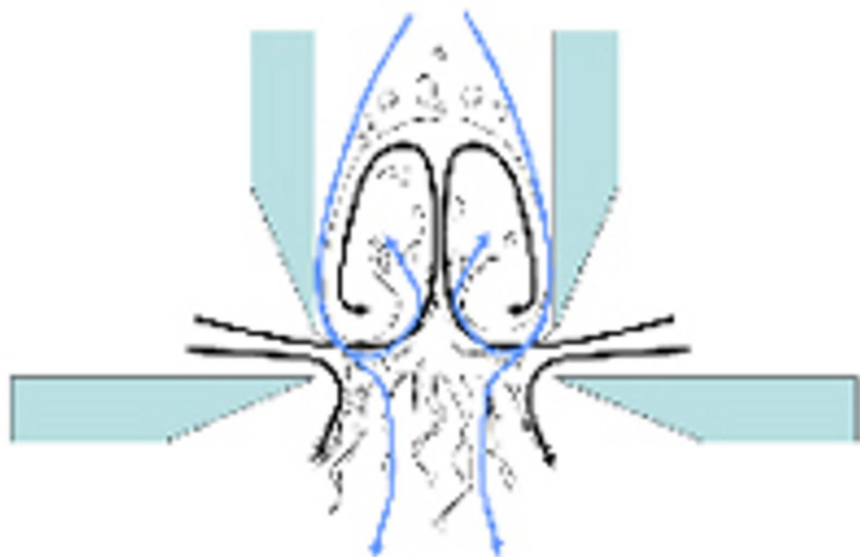
Figure 2 Flow Blurring nebulizer tip showing aerosol creation.
