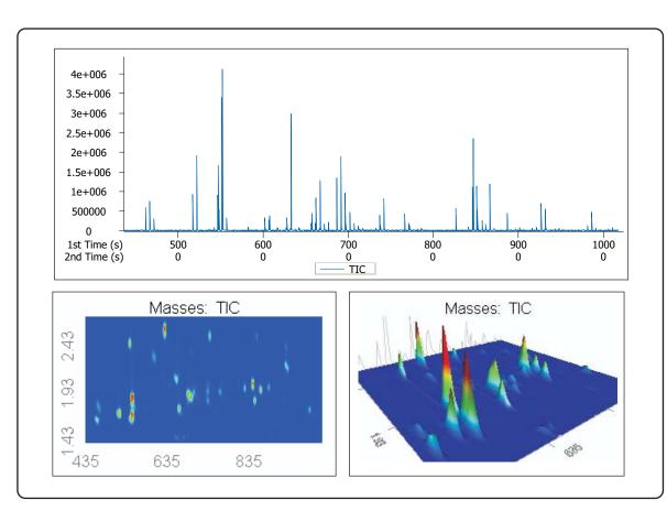
This injection of Hand Soap was analyzed by GCxGC-TOFMS to highlight the capability of the system to display peaks in the second dimension that would not be visible by conventional gas chromatography.
