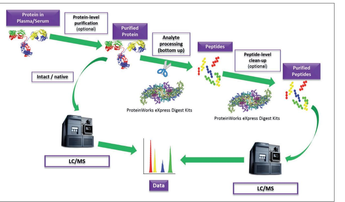
Figure 1: Typical workflows in protein LC-MS.
