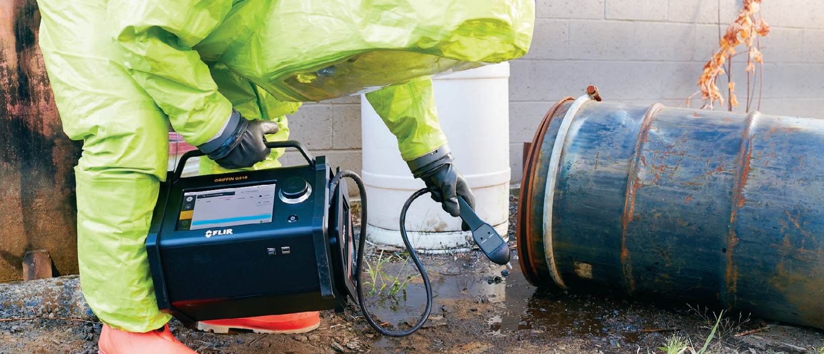
Figure 1 – FLIR Griffin G510 portable GC-MS analyzing a chemical spill in Vapor Survey mode.
