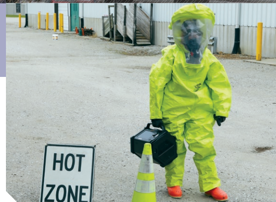
FLIR Griffin G510 Portable GC-MS can be used in the hot-zone while wearing full PPE.
