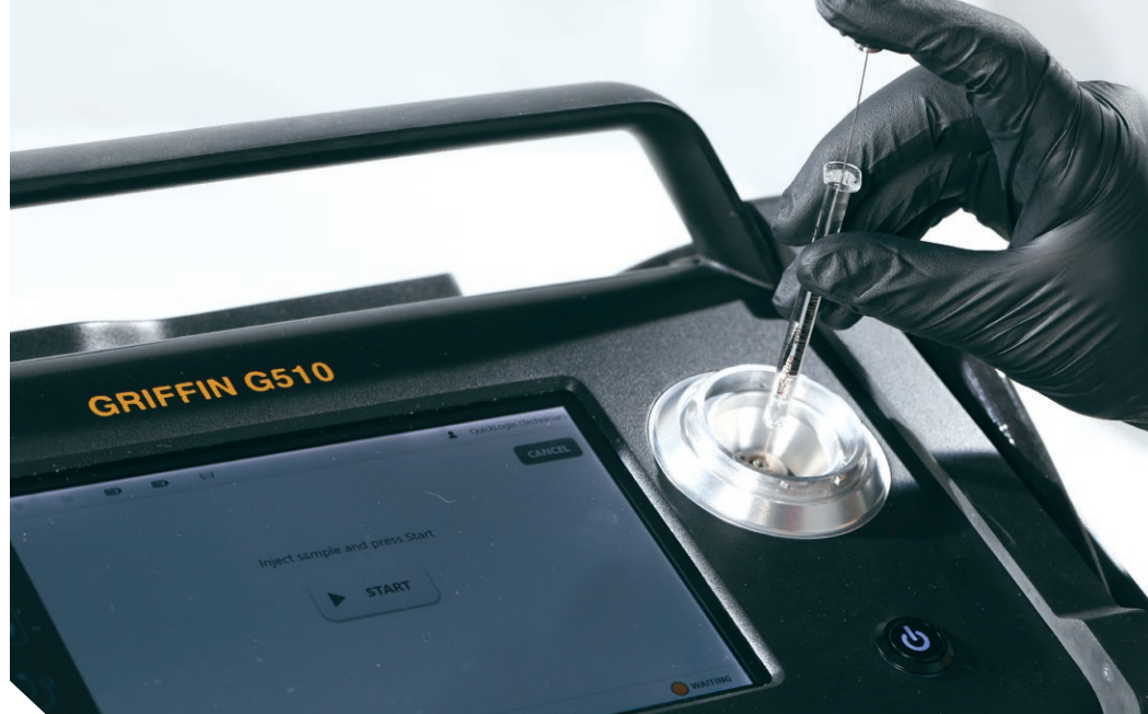
Figure 4 – Syringe injection being performed on the FLIR Griffin G510 portable GC-MS.
